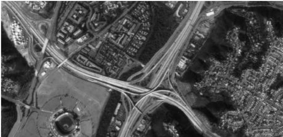
In this 2X (18 x 18 inch) enlargement of the same photograph, at a scale of 1:20,000, 1 inch on the photograph represents 1,666 feet on the ground.
